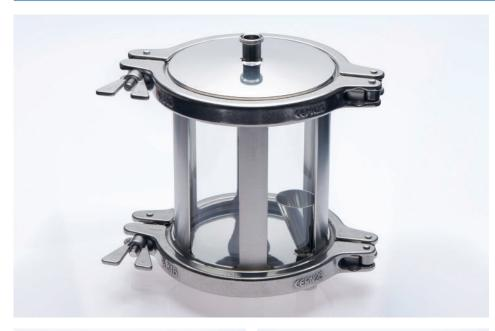
The **CT-Bubble Trap** has been developed to incorporate the best features of the ACL Bubble Trap and the CT-SVFI. The glass/ o-ring/flange end is sealed utilising a sanitary clamp. As there is a mechanical stop, the gasket cannot be overcompressed. The use of a clamp connection reduces the need for tools to assemble or disassemble the bubble trap. Additional seals provide a secondary barrier to prevent the ingress of contaminants to the seal location.
